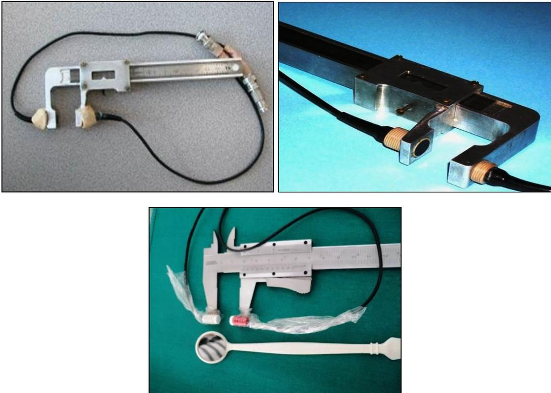
**Fig. 2: Prototype SOS-measurement instrument used in the study.**
